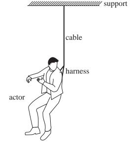
(a) The force on the cable must not cause the material of the cable to reach its yield point.
