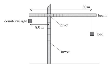
(i) Explain how the counterweight needs to move when the load is moved away from the tower.
